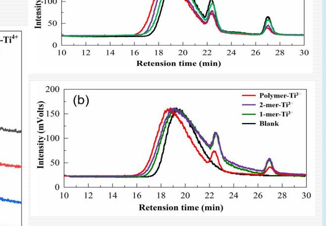
New peaks were identified after crosslinked by PA- Ti<sup>4+</sup>, represent the chelating reaction between PA and Ti<sup>4+</sup> within gelatin film. a gradually increasing gelatin molecular weight after crosslinking treatment. Furthermore, the molecular weight of the gelatin was also affected by the type of the crosslinker, the higher the PD of the PA, the higher the gelatin molecular weight were observed.
