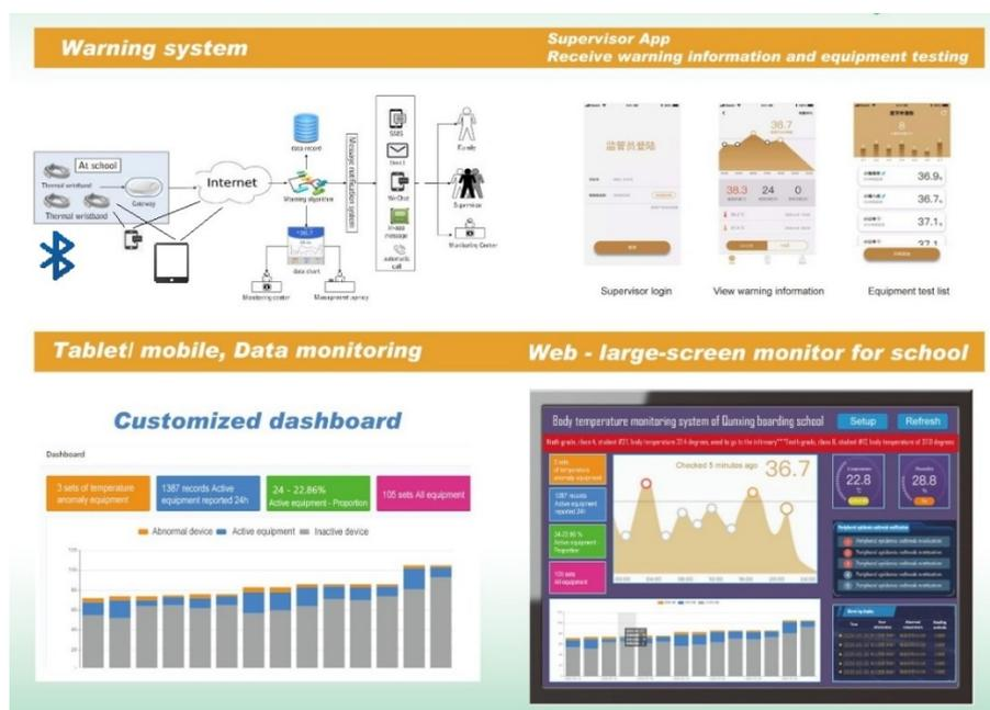
Fig. 2. Outline of the sensor network and images of the software interface.
