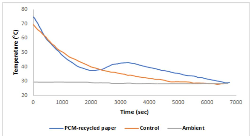
Figure 3. Temperature-time profile of control sample, composite sample and ambience
