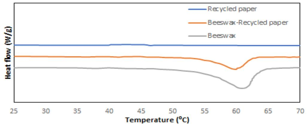
Figure 4. DSC thermogram for melting process
