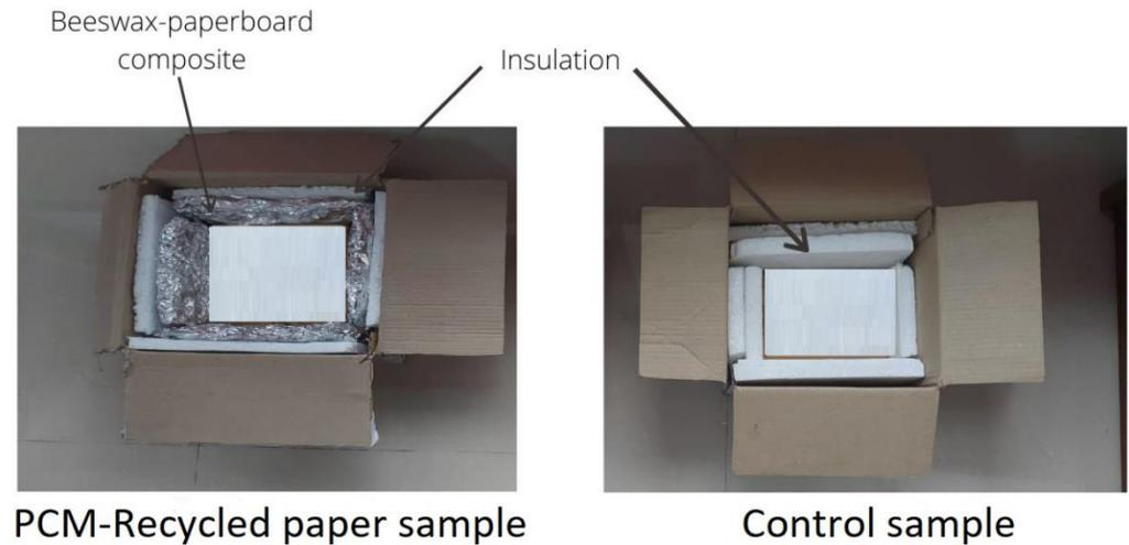
**Figure 1.** Assembly of sample for heat release performance testing
