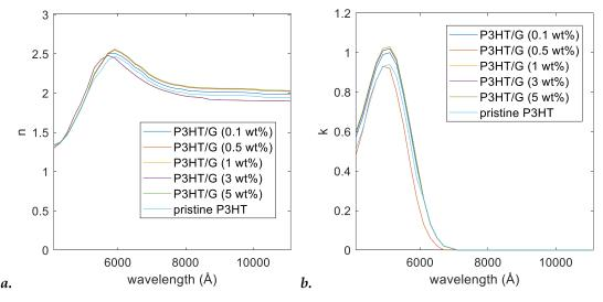
**Figure 2.** Refractive index (a) and extinction coefficient (b) obtained from ellipsometer analysis for P3HT/G nanocomposites with different G loads [3]
