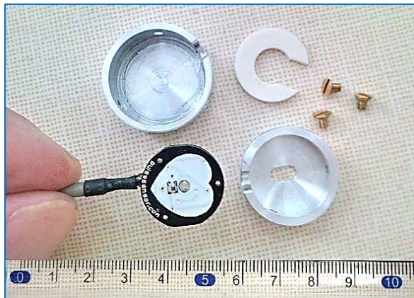
Assembling and aluminum covering of optical Pulse sensor (left) , PPG-PS1 sensor body (middle), PPG-BLE sensor body with Li polymer battery (right).
