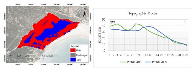
**Figure 2. Left**: Volumetric variation representation of the Valdevaqueros dune, showing loss and gain zones (blue and red) between 2008 and 2015. **Right**: Topographic Profile of the Valdevaqueros dune for 2008 and 2015.
