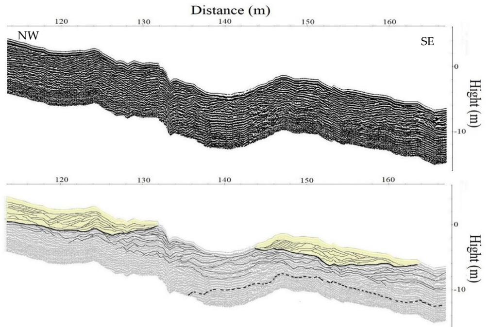
**Figure 4.** Part of the radargram corresponding to the beach-crest transect and its corresponding interpretation.
