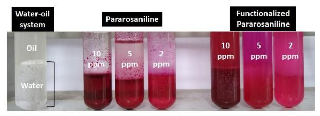
Figure 2. Picture of pararosaniline and functionalized pararosaniline dissolved in a water-oil system at different concentrations.
