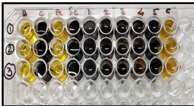
Figure 1. PPA Inhibitory Activity of Various Plant Extracts Using Qualitative Starch Iodide Assay. B: Blank, C: Control, EC: Enzyme Control, SC: Substrate (drug/Acarbose) Control, 1: Pet Ether, 2: Chloroform, 3: Ethyl Acetate, 4: Acetone, 5: Methanol, 6: Water Extract. 3 numbered rows indicate assays done in triplicate.
