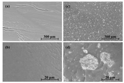
**Figure 1.** SEM images of PBAT (a, b) and PBAT+20%P (c, d) at different magnifications, as representative samples.
