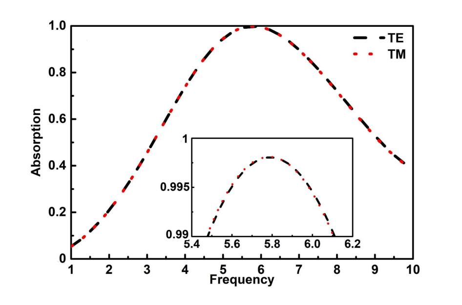
The maximum absorption is 99.8% at 5.79 GHz in the case of TE polarization. Absorption over 99% in a frequency range from 5.48 to 6.1 GHz.
