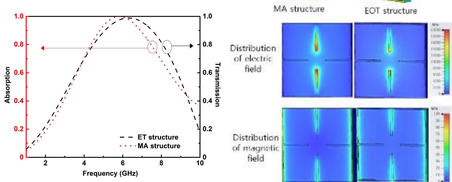
Two spectra very close but the spectrum of transmission broader than that of absorption. The localized electric and magnetic fields on the surface of MA structure seem to be stronger than that those of EOT
