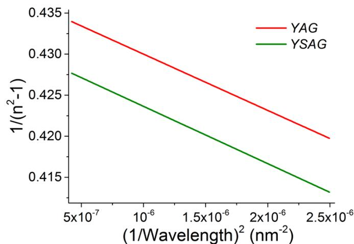
**Figure 2.** Refractive index ( $n$ )–wavelength ( $\lambda$ ) dependence.
