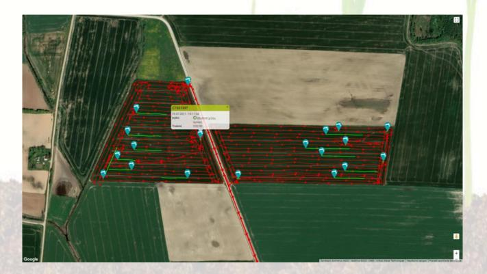
The analysis of the data of the Telemetry system showed that the efficiency of the combine and the reduction of fuel consumption significantly depend on the organization of working processes. The data of the structure working time in Telemetry were showed that the combine devoted from 35 to 57 % of the total day working time to the technological process.
