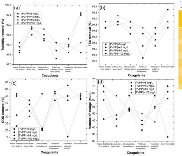
Effect of polyelectrolyte (PVPP) addition in the removal of (a) turbidity, (b) TSS, (c) COD, (d) volume of sludge. CFD operational condition ( $[COD]_0$  = 2145 mg O<sub>2</sub>/L, turbidity = 296 NTU, TSS = 750 mg/L, temperature 298 K, sedimentation time 12 h).
