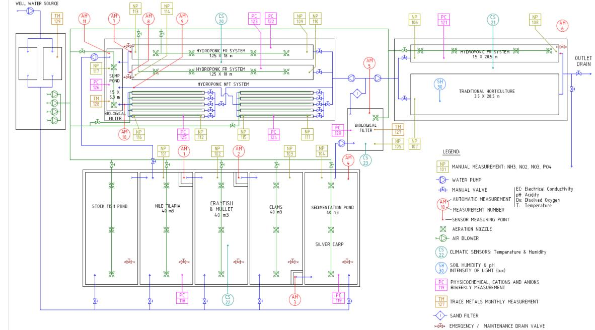
Figure 2: Blueprint of the experimental greenhouses (water flow-blue; airflow-green; drainage system-dark red).
