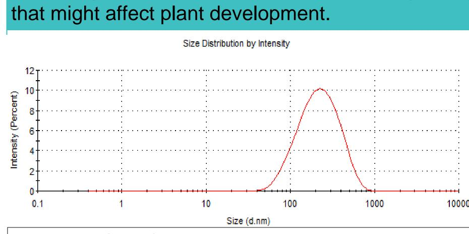
**Fig. 1.** The OMV Serratia sp. diameter were analyzed using the DLS intensity-weighed distribution (Zetasizer, Malvern).
