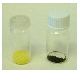
Figure 1: g-SILLPs supported gold species before and after reduction: left, Au(III) supported; right, Au(0) supported.
