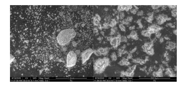
Scanning Electron Microscopy (SEM) images of ferrocene (100 and 500x).
