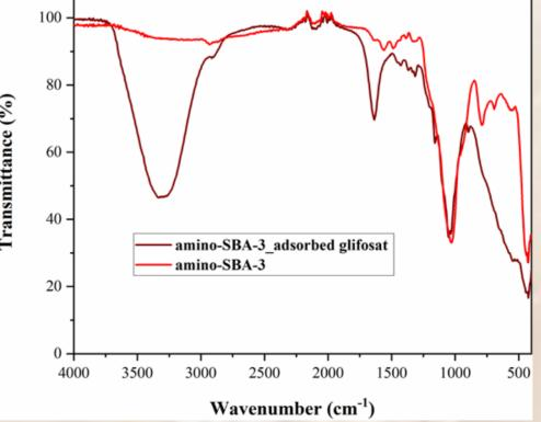
Amino-SBA-3 FTIR spectrum after N-(phosphonomethyl)glycine adsorption
