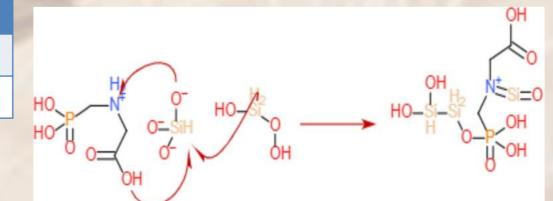
Potential mechanism for the interaction between amino-SBA-3 and glyphosate
