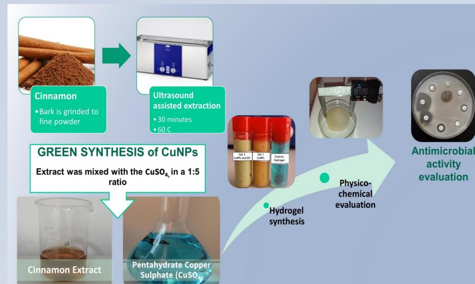
Figure 1. Formulation of a multifunctional nanocomposite hydrogel based on natural polysaccharides, biogenic copper nanoparticles and essential oils
