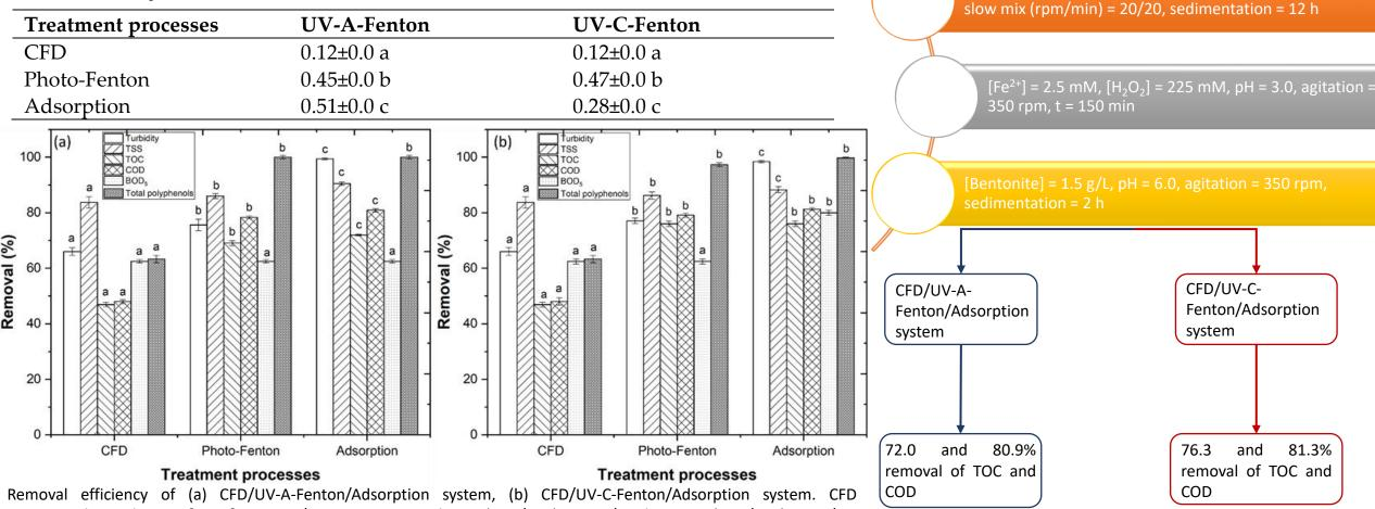
Removal efficiency of (a) CFD/UV-A-Fenton/Adsorption system, (b) CFD/UV-C-Fenton/Adsorption system. CFD operational conditions: [PVPP] = 0.5 g/L, pH = 6.0, rapid mix (rpm/min) = 150/3, slow mix (rpm/min) = 20/20, sedimentation = 12 h. Photo-Fenton operational conditions:  $[Fe^{2+}] = 2.5 \text{ mM}$ ,  $[H_2O_2] = 225 \text{ mM}$ , pH = 3.0, agitation = 350 rpm, t = 150 min. Adsorption operational conditions: [Bentonite] = 1.5 g/L, pH = 6.0, agitation = 350 rpm, sedimentation = 2 h.
