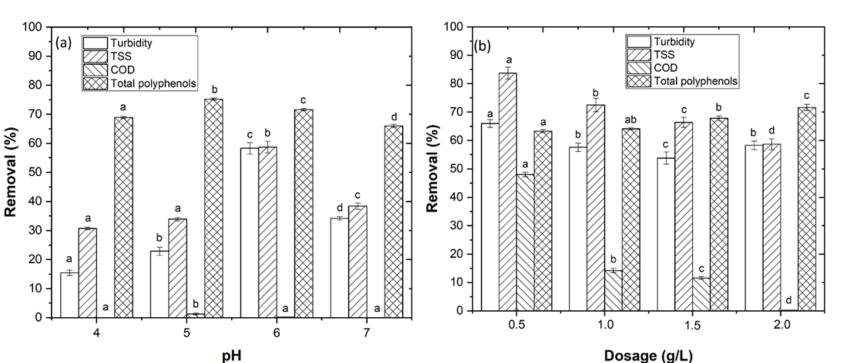
Optimization of (a) pH (4.0 - 7.0) under the following conditions: [PVPP] = 2.0 g/L, rapid mix (rpm/min) = 150/3, slow mix (rpm/min) = 20/20, sedimentation = 12 h; (b) PVPP dosage (0.5 - 2.0 g/L) under the following conditions: pH = 6.0, rapid mix (rpm/min) = 150/3, slow mix (rpm/min) = 20/20, sedimentation = 12 h. Columns with different letters are significantly different.
