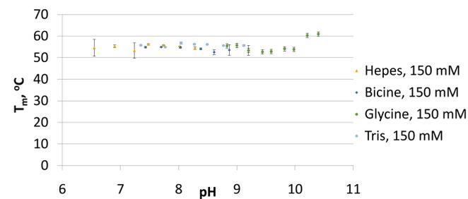
Figure 4. Graph illustrating the dependence of psCA2 melting temperature ( $T_m$ ) on ambient pH values in different buffers.
