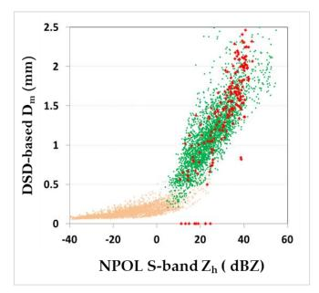
**Figure 3.** Same as panel (b) of Figure 1 but with experimental data (red points) superimposed from an event over Delmarva peninsula (outer-rainbands of category-1 Hurricane Dorian on 6 September 2019), shown as red points, with Dm values from 3-min DSD disdrometer measurements and Zh from the NPOL S-band radar measurements over the disdrometer site.
