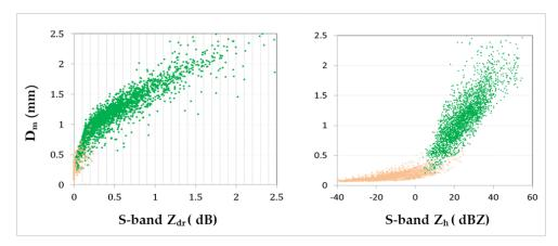
Figure 1. Scattering simulations using DSD measurements. DSD-based  $D_m$  versus (a)  $Z_{dr}$  and (b)  $Z_h$  both at S-band. The orange points represent the measurements in stratacumulous drizzle (aircraft) and the green points represent measurements from ground-based disdrometers in Greeley, Colorado, and Huntsville, Alabama.
