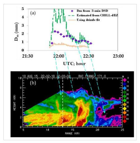
**Figure 6.** (a) D<sub>m</sub> comparisons for another event (10 August 2015) in the same way as Figure 5. (b) CHILL S-band RHI scan taken along the azimuth angle of the disdrometer site (at 13 km range, marked with a dashed white line) at 22:02 UTC. The blue arrows point to the different rain types as they passed over the disdrometer site corresponding to the UTC in panel (a).
