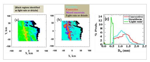
**Figure 7.** (a) 500 m by 500 m gridded data (dBZ) constructed from NPOL volume scan during an embedded line convection event over Delmarva peninsula on 30 April 2021 (see [20] for details). (b) Rain-type classification (retrieved DSD-based) for stratiform, convective, and mixed rain types and regions identified as light-rain marked in black. (c)  $D_m$  histograms estimated for the regions identified as light rain compared with those for stratiform and convective rain.
