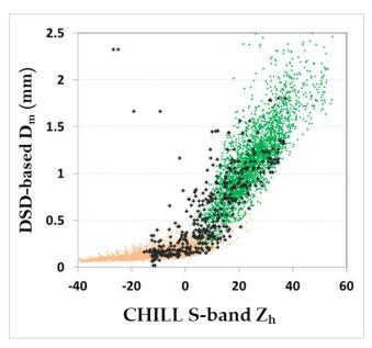
**Figure 2.** Same as panel (b) of Figure 1 but with experimental data (black points) superimposed from an event on 17 April 2015 at Greeley, Colorado, with Dm values from 3-min DSD disdrometer measurements and Zh from the CSU-CHILL S-band radar measurements over the disdrometer site.
