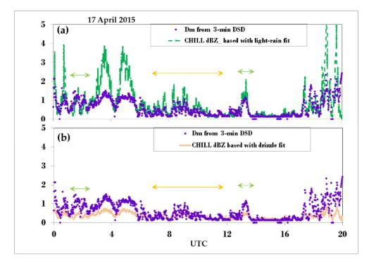
Figure 5.  $D_m$ 's from 3-min DSDs (purple) for the long duration event on 17 April 2015 and  $D_m$  estimates from the CSU-CHILL S-band radar dBZ over the disdrometer site using the fitted equation for (a) light-rain (green points) and (b) drizzle (orange). The orange and the green arrows represent the time intervals when the drizzle-fit and the light-rain fit yield better agreement with the DSD-based  $D_m$ 's respectively.
