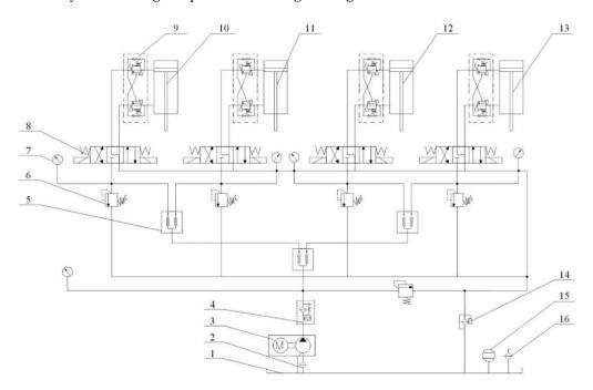
1 oil tank; 2 filter; 3 oil pump motor unit; 4 pressure oil filter; 5 diverter valve; 6 relief valve; 7 pressure gauge; 8 electromagnetic reversing valve; 9 balance valve; 10 crane hydraulic cylinder group; 11 Front outrigger hydraulic cylinder group; 12 Middle outrigger hydraulic cylinder group; 13 Rear outrigger hydraulic cylinder group; 14 Oil return filter; 15 Liquid level gauge; 16 Air filter
