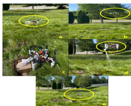
Figure 5. Drone taking off from the initial point (a), drone en route to be landed landmark (b), drone landmark doing excavation autonomously (c), Dumping the excavated soil (d), and the drone arrived back after the excavation operation (e).
