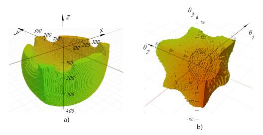
**Figure 2.** Workspace virtual model of the delta robot: a) in (x, y, z) coordinates, b) in coordinates  $\theta(i)$
