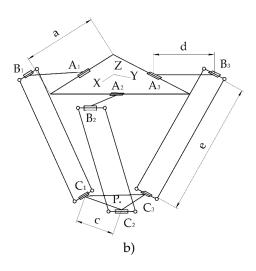
**Figure 1.** Robotic system: a) 3D model: 1—body, 2—DeLi manipulator, 3—dispensing head, 4—dispenser tip, 5—robot manipulator, 6—base of the robot manipulator, 7—workspace, 8—trolley, 9—tray for consumables, 10—rack with test tubes, b) delta-robot structure
