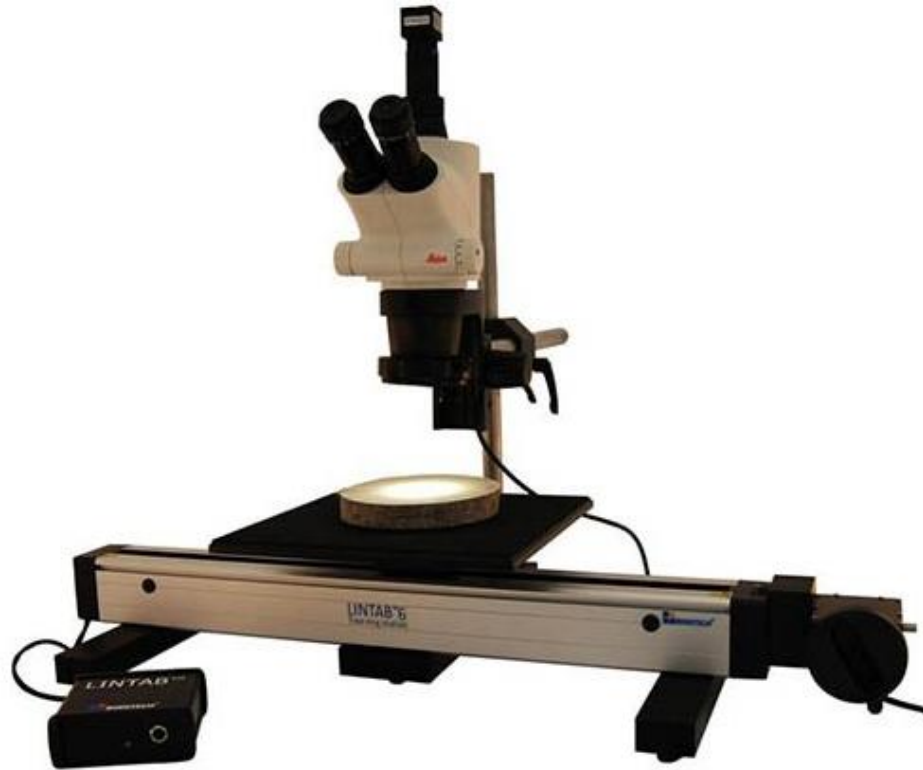
LinTab™ 6 tree-ring width measuring instrument (Rinntech, Heidelberg, Germany)
