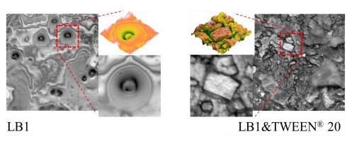
**Figure 2.** Images of surface structures based on superlattices of latex particles LB1 and their mixture with nonionic surfactant TWEEN® 20 obtained in an optical microscope. The 3D images (built using the Gwyddion software environment) of the enlarged areas are shown for illustrative purposes only to more clearly emphasize the symmetry of the optical structure of the image.
