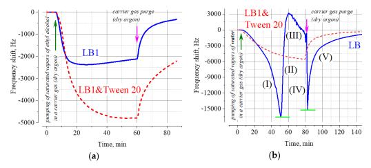
**Figure 1.** The typical responses of QCM transducers modified with LB1 and a mixture of LB1 with TWEEN® 20 when saturated ethyl alcohol (a) or water (b) vapors is pumped over their surface.
