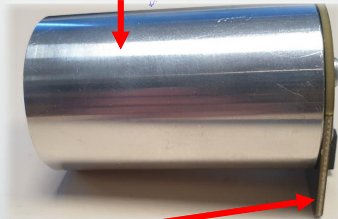
Metal Tube used as field of view limiter
