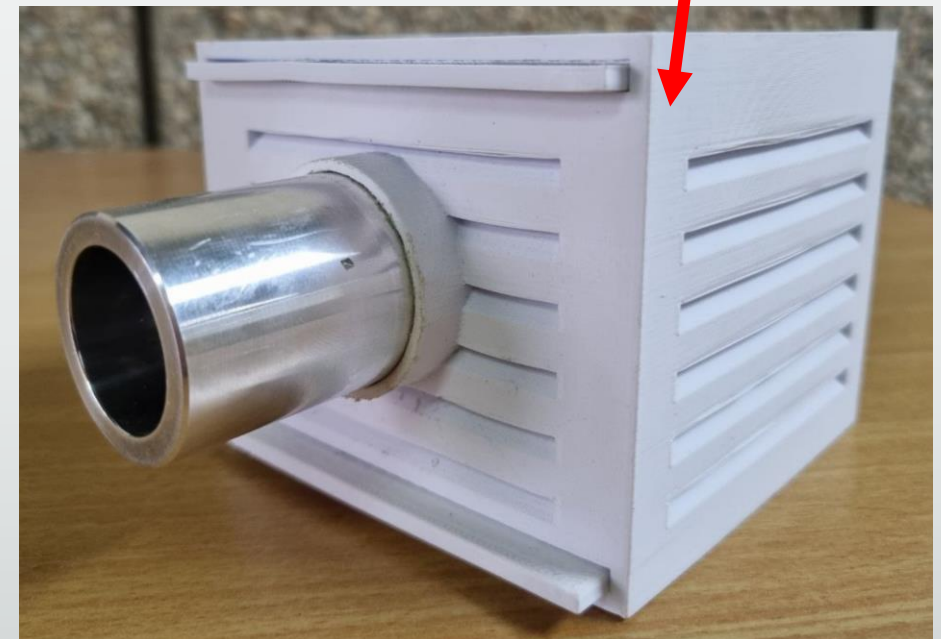
Air Temperature Box with the Digital-TMOS, Microcontroller and additional environmental sensors
