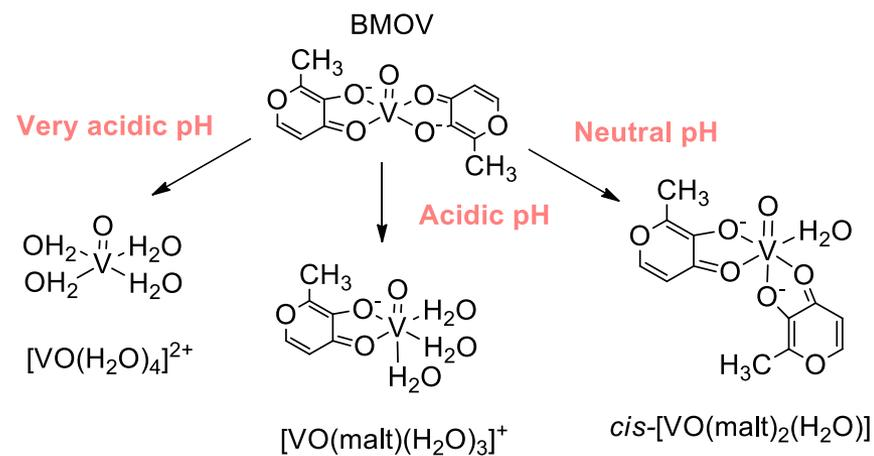
Structure of BMOV and its possible transformations in aqueous solution
