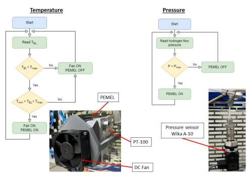
Figure 3. Control algorithms for temperature and pressure. Equipment involved.
