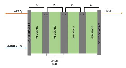
Figure 1. Structure and operation of PEMEL.
