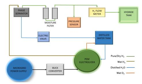
Figure 2. PEMEL hydrogen generation system.
