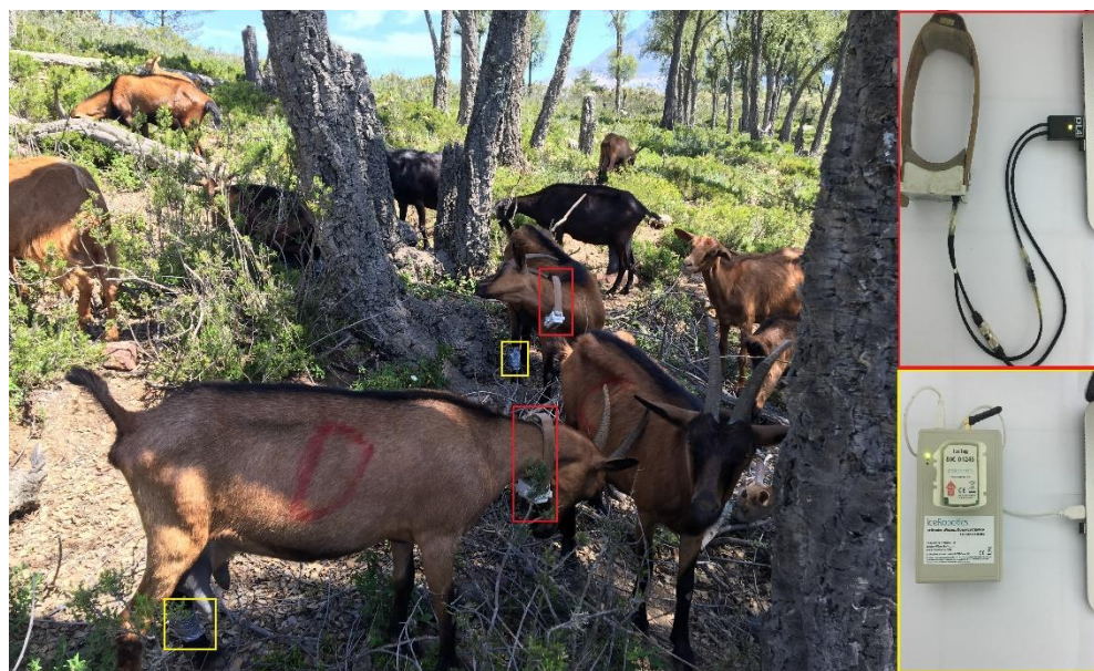
Figure 1. Alpine goat equipped with a GPS collar on the neck (red) and leg sensor positioned on the rear left leg (yellow) in the studied forest rangeland of Northern Morocco.
