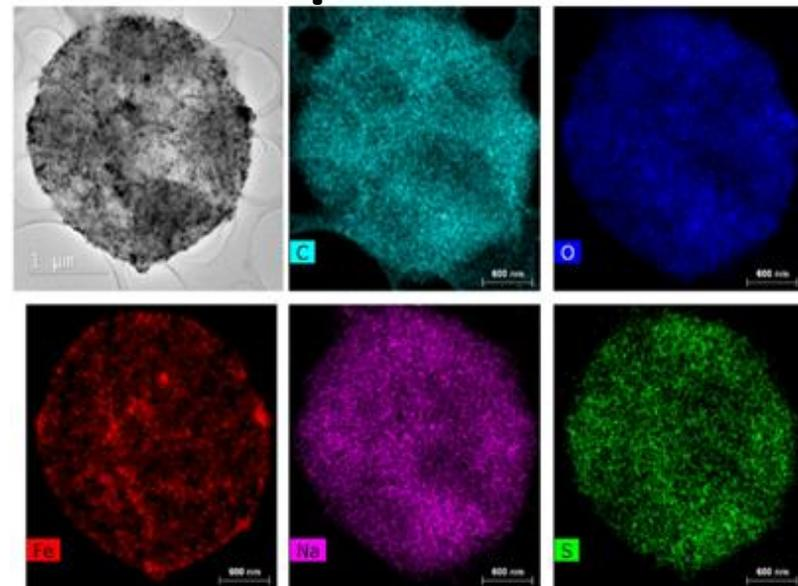
TEM image of microcapsules and element mapping
