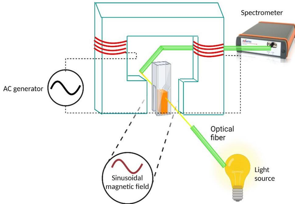
The *in situ* release of TRITC-dextran from the microcapsules was evaluated by measuring the optical density during the influence of magnetic field. For this, magnetic field generator with built-in light source and spectrometer were used. The scheme of the set-up is presented in Figure.
