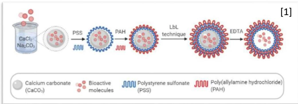
Microcapsules were prepared by the layer-by-layer method.
