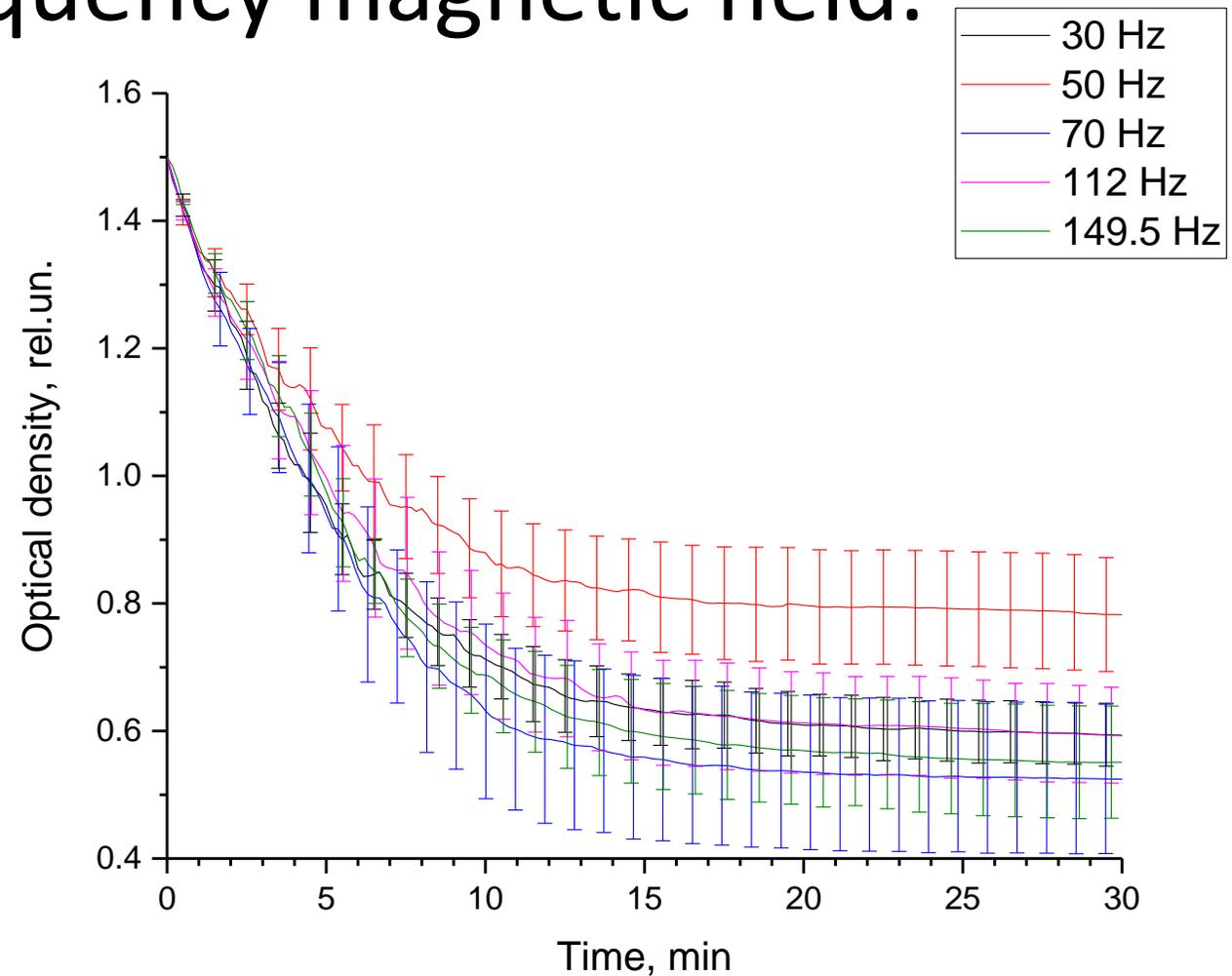
Optical density curves for suspension of capsules loaded with TRITC-dextran under exposure of LFMF with different frequency
