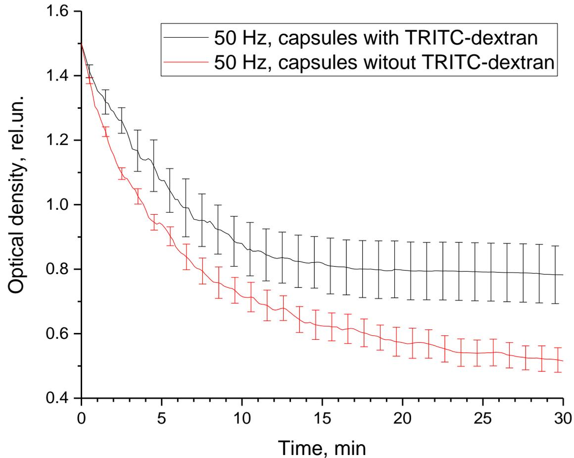
Optical density curves for suspension of capsules loaded with TRITC-dextran and for control sample under exposure of LFMF
