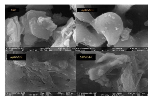
Figure 4. The SEM images of CaO and Ag@CaO(1), Ag@CaO(2), Ag@CaO(3) nanocomposite.
