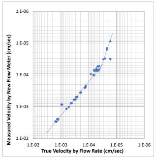
Figure 2. Correlation between True Velocity and Measured Velocity
