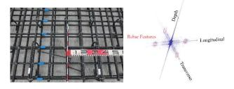
radar data. As rebars being placed in a certain spacing, peaks appear on longitudinal and transverse axes in the frequency domain. Focusing on a surface that includes rebar vertex in the filtered data and by a peak detection method, 3D rebar mesh was produced.
