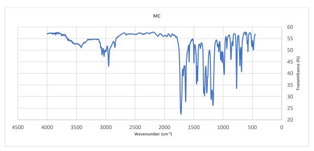
Figure 2. The IR spectrum of methyl cinnamate.
