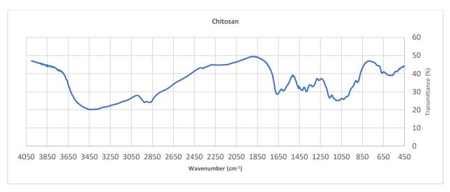
Figure 4. The IR spectrum of chitosan. .
