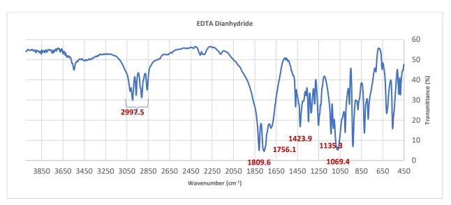
Figure 1. The IR spectrum of EDTA dianhydride.
