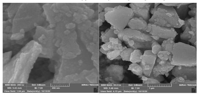
Figure 3. FE-SEM images of g-C<sub>3</sub>N<sub>4</sub>@L-arginine.
