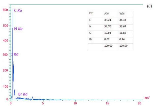
Figure 2. EDX spectra of a) g-C<sub>3</sub>N<sub>4</sub> nanosheets, b) modified g-C<sub>3</sub>N<sub>4</sub>, and (c) g-C<sub>3</sub>N<sub>4</sub>@L-arginine.
