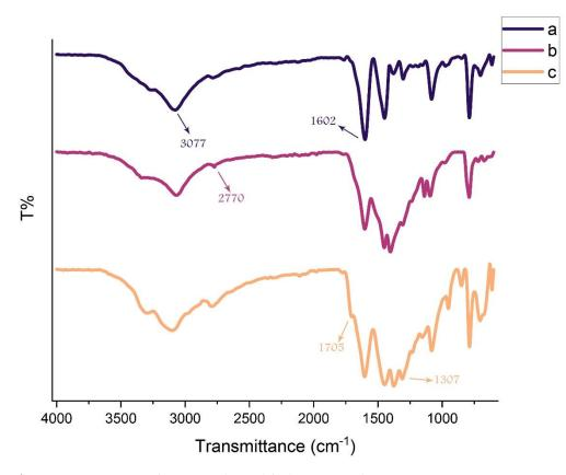
Figure 1. FT-IR spectra of a) g-C<sub>3</sub>N<sub>4</sub>, b) modified g-C<sub>3</sub>N<sub>4</sub>, and c) g-C<sub>3</sub>N<sub>4</sub>@L-arginine.
