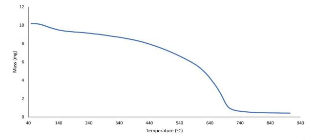
Figure 5. TGA spectrum of g-C<sub>3</sub>N<sub>4</sub>@L-arginine.
