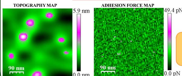
The use of **flexible spacers** to attach the ligand at the tip removes non-specific interactions improving the measurement of the specific interaction forces. Operating in JM, topography and adhesion images are obtained simultaneously. When operating JM in repulsive regime, adhesion images become MRI images. Images obtained using PEG-maleimide-Fd modified tips [2].
