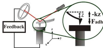
**Single Molecule Force Spectroscopy (SMFS)** measures the interaction forces between a ligand molecule attached to the AFM tip and a receptor molecule immobilized on a surface. At a given loading rate hundreds of force-distance (Fz) curves are taken (left). Rupture events are processes of stochastic nature and their analysis allows calculating the unbinding force corresponding to a single complex and other parameters of the transition state.
