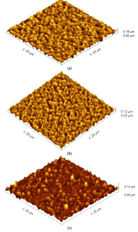
**Figure 1.** Topography images of chitosan samples deposited on glass slides: (**a**) pristine chitosan (reference); (**b**) one layer of (0.01 wt% GO blended with chitosan); (**c**) Three layers of (0.01 wt% GO blended with chitosan).
