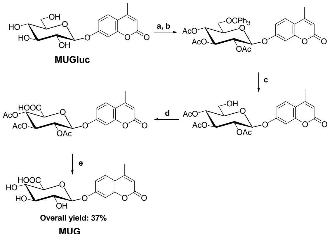
**Scheme 1** a) Ph<sub>3</sub>CCl, pyridine, 90 °C, 5 h. b) acetic anhydride, r.t., 24 h, 73%. c) I<sub>2</sub>, MeOH, benzene, 65 °C, 24 h, 92%. d) NaOCl, TEMPO, NaBr, NaHCO<sub>3</sub>, Bu<sub>4</sub>NBr, CH<sub>2</sub>Cl<sub>2</sub>-H<sub>2</sub>O, 0 °C, 3h, 68%. e) Ba(OMe)<sub>2</sub>, MeOH, 0-5 °C, 24 h, 85%.
