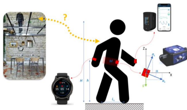
Figure 3. Experimental setup for the analysis of human comfort based on kinematic and biometric parameters (detail photo reproduced from [7] under the terms and conditions of CC-BY license agreement).
