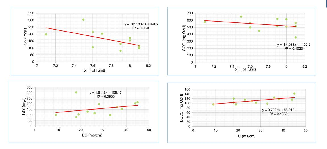
Scatter plots showed positive linear relationships between total suspended solids (TSS) and SO4, total suspended solids (TSS) and EC, and BOD5 and EC. Nonetheless, both TSS and COD show negative linear relationships with ph.
