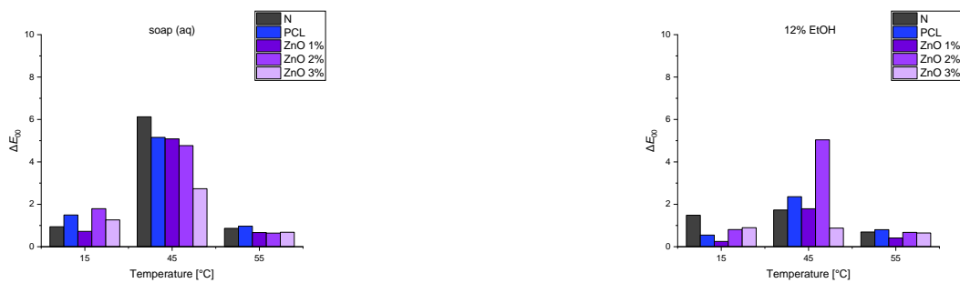
Figure 2. Total colour difference (TCD) between two states (measured at 15, 45 and 55 °C) for uncoated and coated TC print before and after exposure to different chemical agents.
