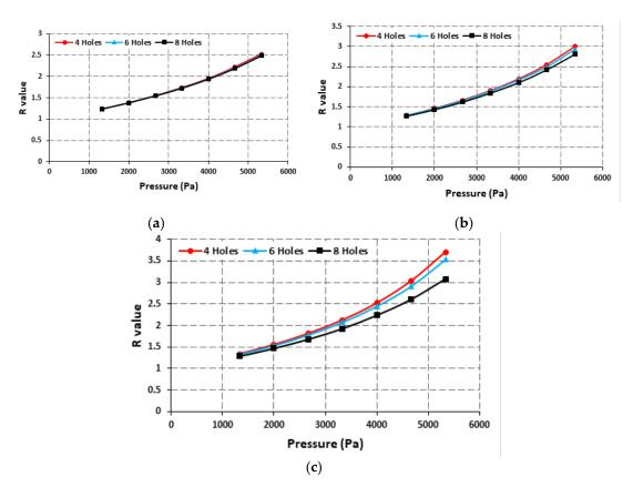
**Figure 4.** Effect of number of holes and hole size on the R value; (a) Hole size of 1 mm; (b) Hole size of 1.5 mm; (c) Hole size of 2 mm.
