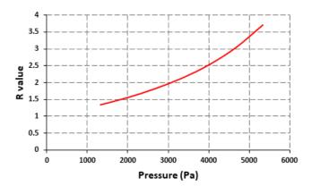
**Figure 5.** R value at different IOP values for the design with 4 holes of 2 mm diameter.
