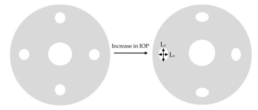
**Figure 1.** Schematic of proposed lens design, the shape of the holes changes in response to a change in IOP.
