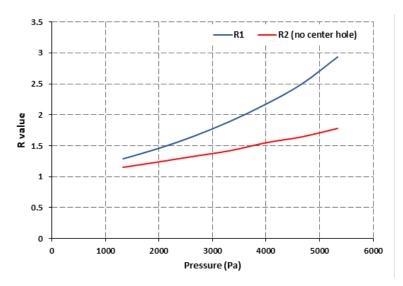
Figure 3. Change in R value with applied pressure for the designs with and without center hole.
