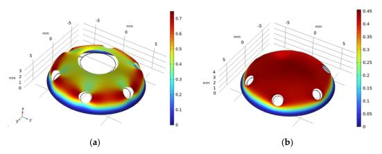
Figure 2. Effect of central hole on the deformation of the lens (a) Lens with a center hole; (b) Lens without a central hole.
