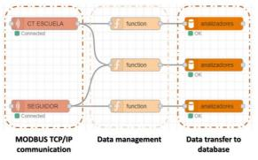
Figure 3. Node-RED program for data acquisition and transfer to database.
