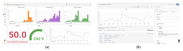
**Figure 5.** Graphical appearance and operation of Grafana. (a) Dashboard and synoptics overview. (b) Graph configuration tab overview.
