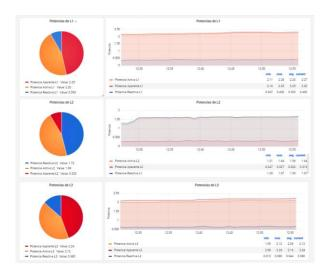
Figure 8. Active, reactive, and apparent powers per line.
