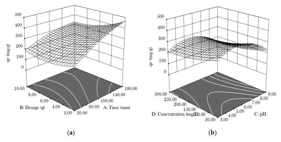
Figure 1. The 3-D surface plots of Zn (II) adsorption (a) dosage and Time, (b) concentration and pH.
