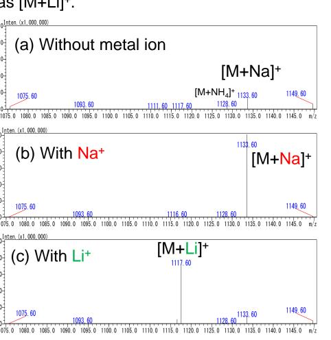
Figure 2 Multi spectra of CTX1B by different mobile phases (SIM).
