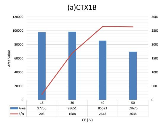
Figure 3 The relationship between the CE and the peak area or S/N.
