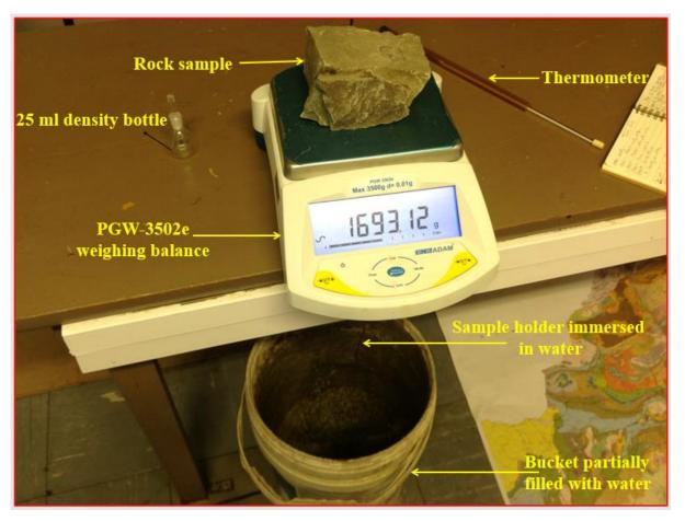
Figure 3. Photo demonstrating the use of Archimedes' Principle in rock samples measurement.
