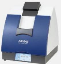
Camag visualizer: ex 254 and 366 нм, measurement – photo camera 3. Absorption/reflectance in visible light
