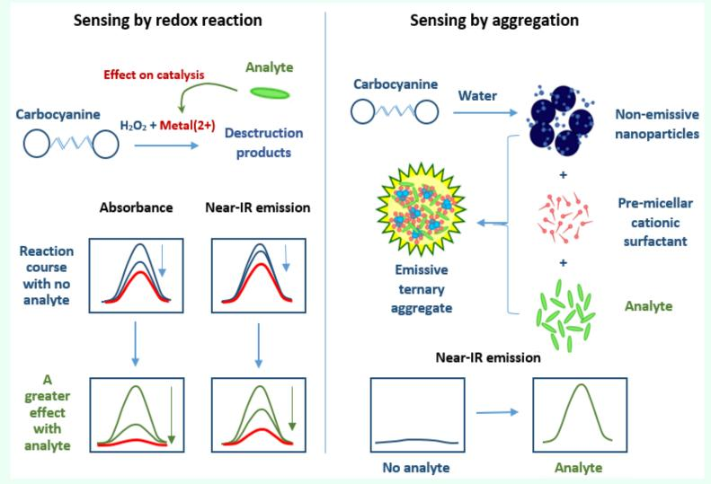
**Mechanism 1**. The analyte changes the rate of the dye oxidation reaction  $\rightarrow$  fluorescence fading, color change.
